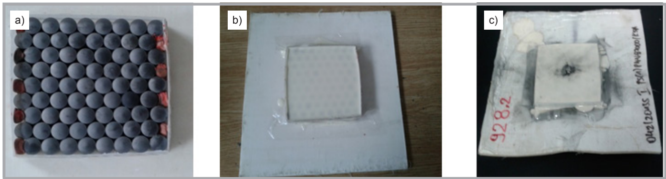
Figure 9. Hybrid ceramic - multi-layered UHMWPE composite armour based on cylindrical ceramic: sample without polyurethane (a), with polyurethane (b), after ballistic tests carried out in accordance with the requirements of PN-V-87000:2011 [33] using a single impact with a 7.62×51 mm AP bullet (c).
