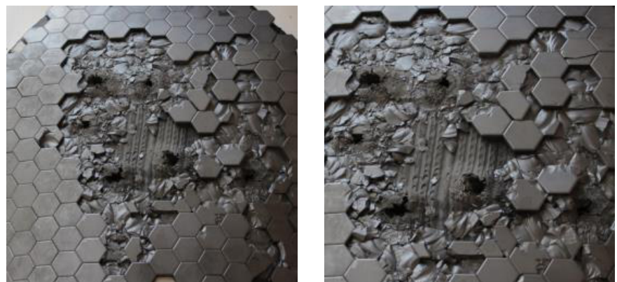
Figure 5. Surface of the hybrid ceramic - multi-layered UHMWPE composite armour after ballistic testing by the multi-hit procedure using 5.56×45 mm SS109.
