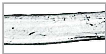
Figure 5. Longitudinal section of the ‘sisal’ fibre - 500×.
