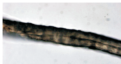
Figure 4. Longitudinal section of the Bactris setosa fibre - 500×.
